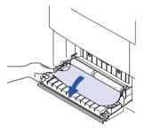
3. If the paper did not come out easily, open the Top Cover and open the Pressure Release Tabs.
